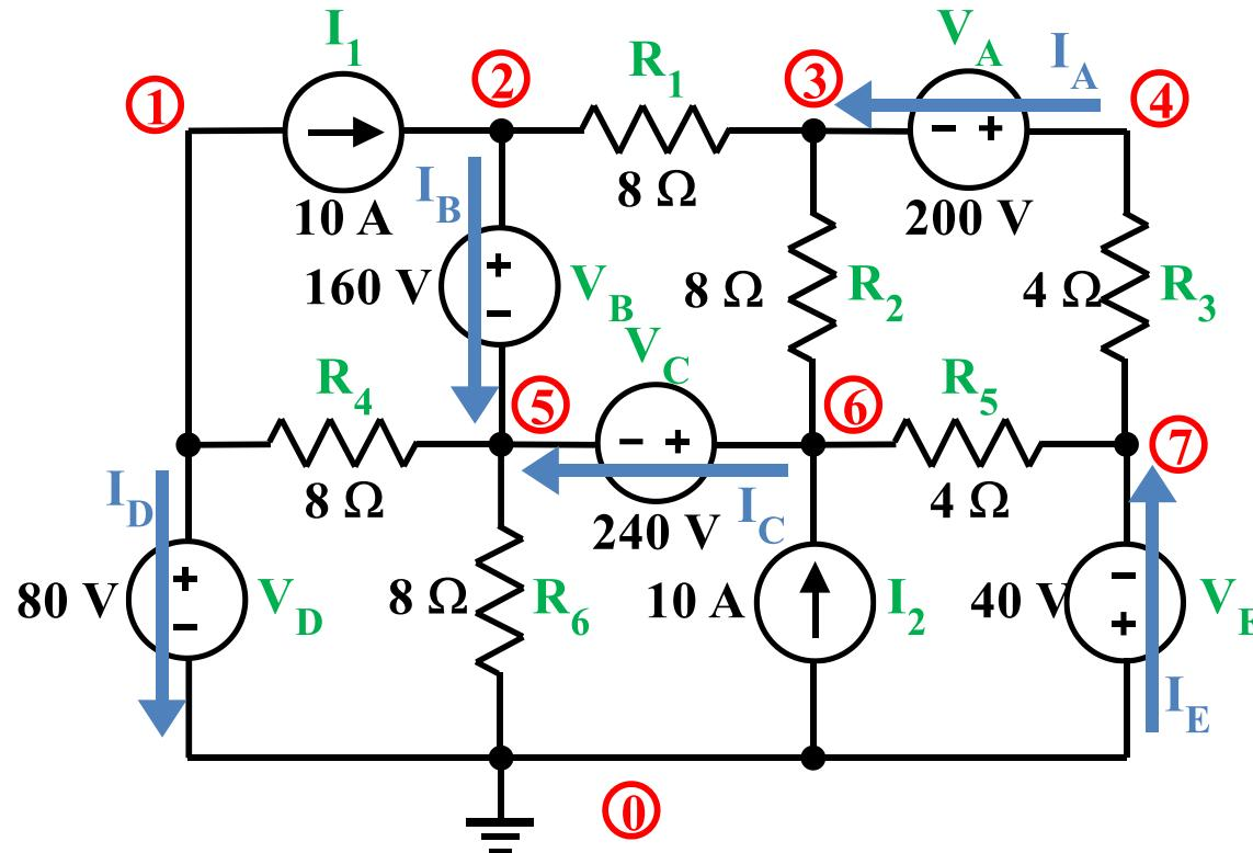
Write a KCL equation at each node (except the reference node), with independent current sources on the right-hand side. Currents leaving the node are taken as positive.
